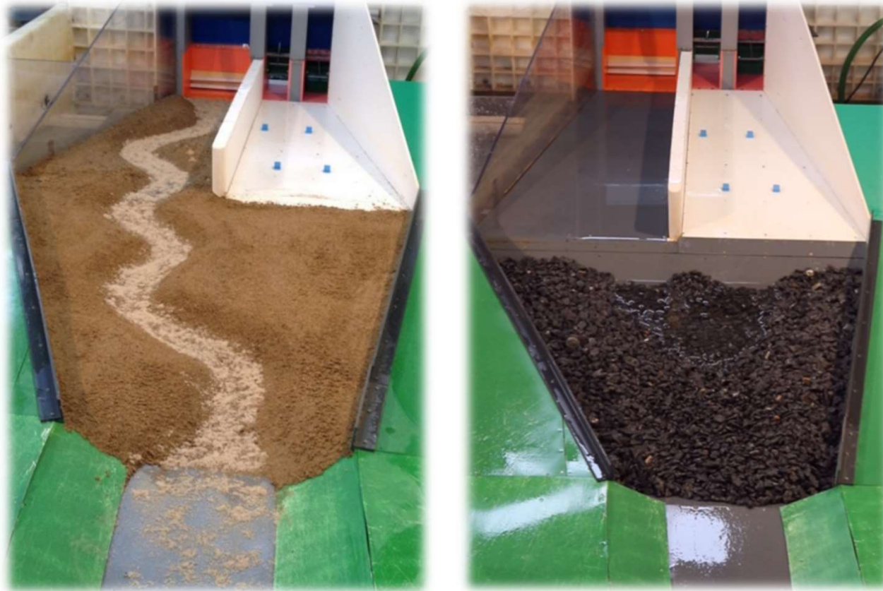
Situation before the experiments (left) and after the experiments with Q_{10,000} (right).
